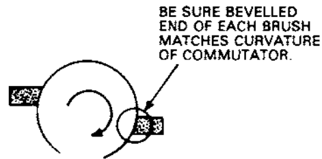
Figure 6-11. Proper Insertion of Brushes
